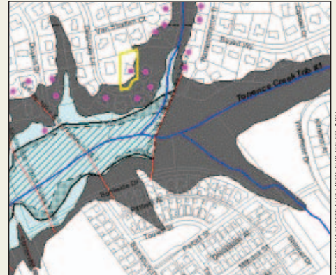
FEMA Floodplain map (light blue) and future Community floodplain (dark gray), Charlotte-Mecklenburg County, NC
